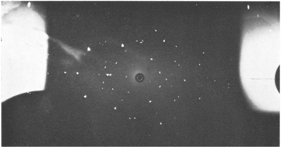
2c Single crystal adherent (111) deposit, substrate temperature 450° C.
